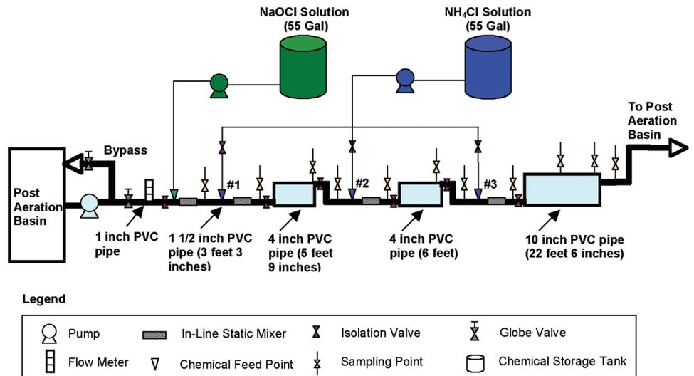
Figure 2. Facility Sequential Chlorination Pilot Plant Schematic
