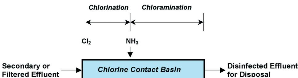
Figure 1. Sequential Chlorination Disinfection
