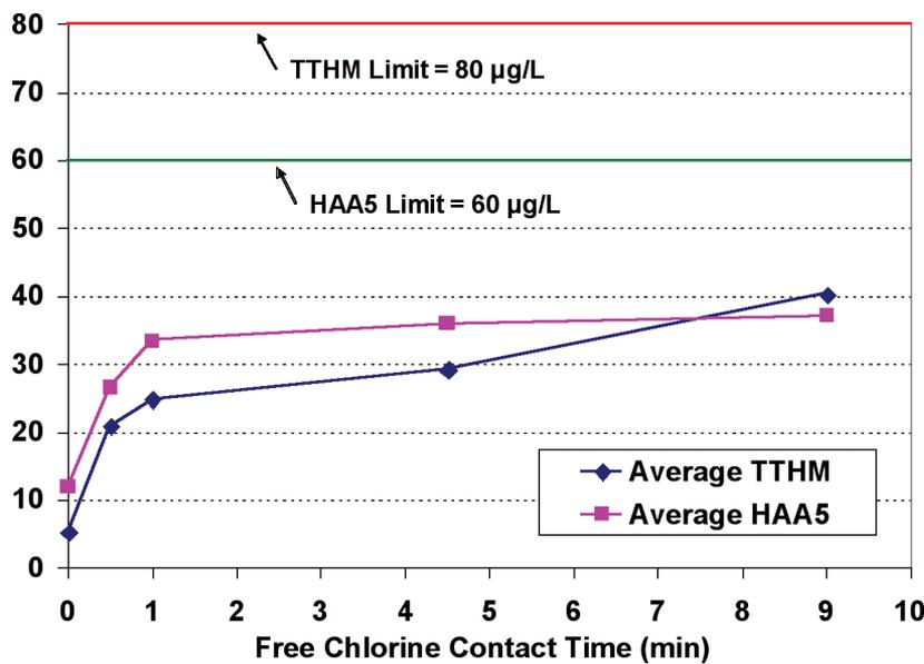
Figure 4. Effect of Free Chlorine Contact Time on DBP Formation
