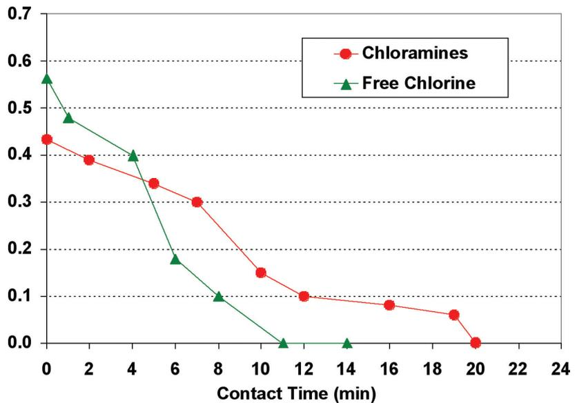
Figure 5. Total Residual Chlorine Decay Test Results—TREEO Sample
